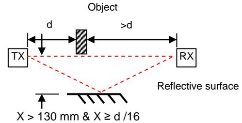
$X$  is minimum distance between the light and the reflective surface. The closest distance of TX or RX to the object approaching the light curtain is  $d$ .
